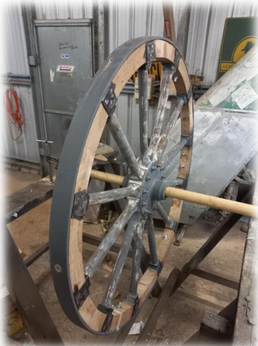
Both wheels required new retaining collars and pins to be made.
