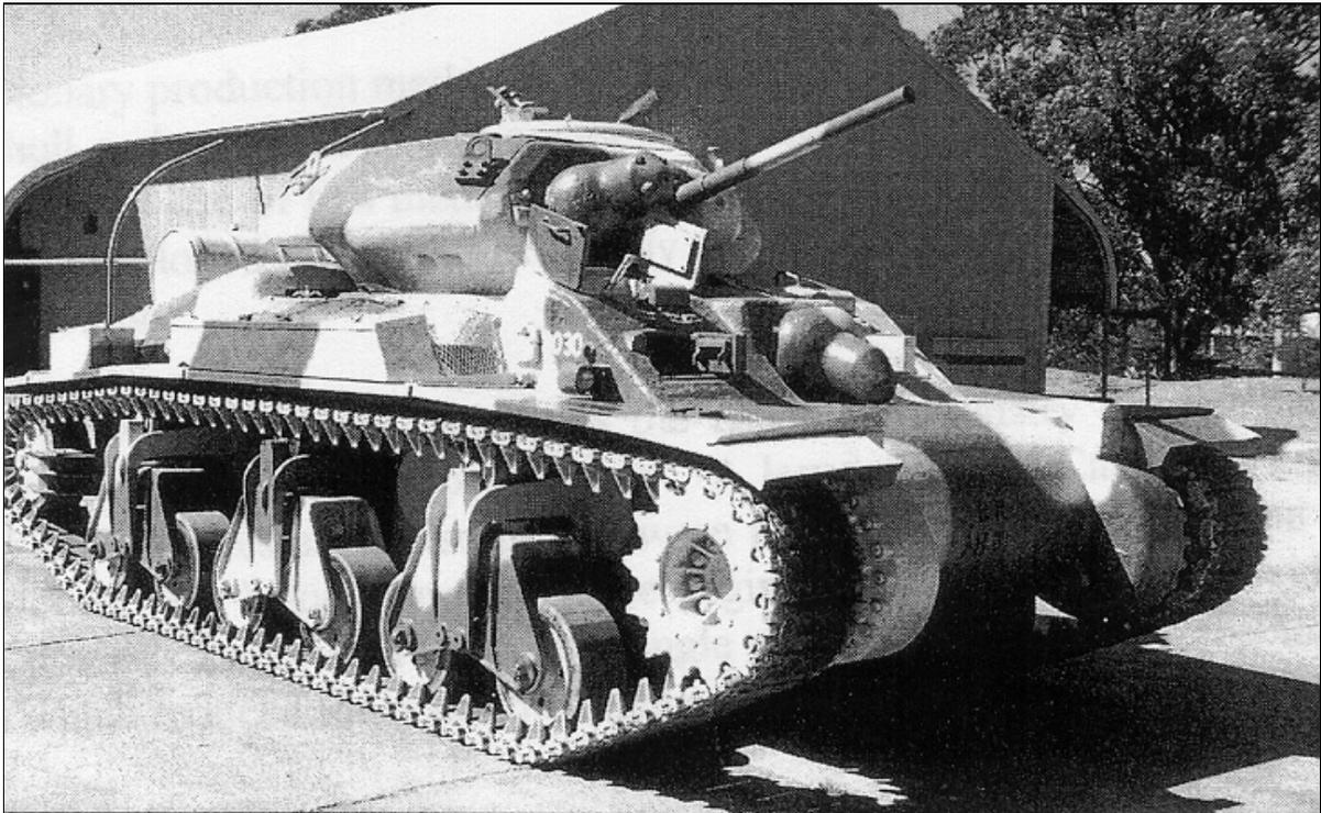
The pilot model of the Sentinel was completed in March 1942 and by August 1942, the first production tank was completed in the NSW Railway Workshops. The first Sentinel Mk I weighed 26 tons, mounted a 2-pr (40 mm) gun and two Vickers machine guns. The frontal armour was 65 mm and the vehicle achieved a top speed of 48 km/h.
